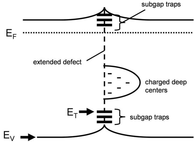
FIG. 1. Illustration of subgap traps at characteristic energy level  $E_T$  compared to the band edge level  $E_V$ . Here the traps occur at an extended defect where the band bending further raises  $E_F$ . Minority carriers trapped at  $E_T$  may participate in the dominant recombination process.
