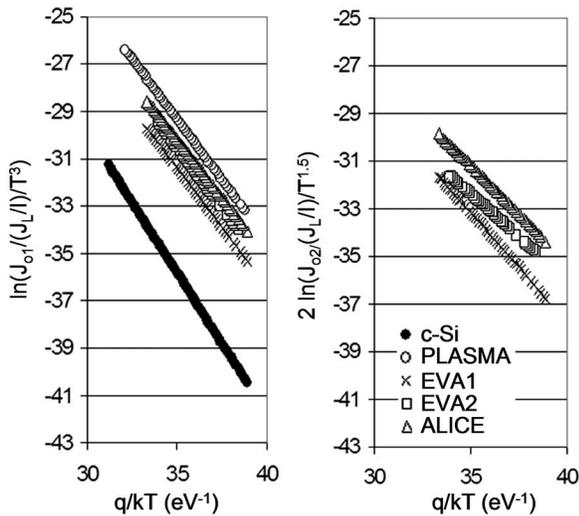
FIG. 4. Arrhenius plots of  $J_{o1}/(J_L/I)$  and  $J_{o2}/(J_L/I)$  of the poly-Si solar cells.  $J_{o1}/(J_L/I)$  for a single-crystal silicon wafer solar cell is also shown for comparison.
