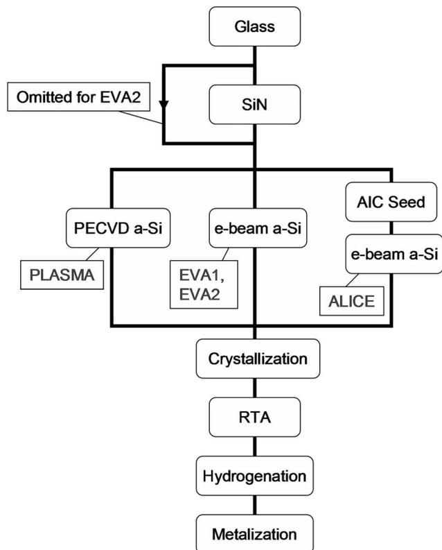
FIG. 2. Process sequence of the poly-Si solar cells.
