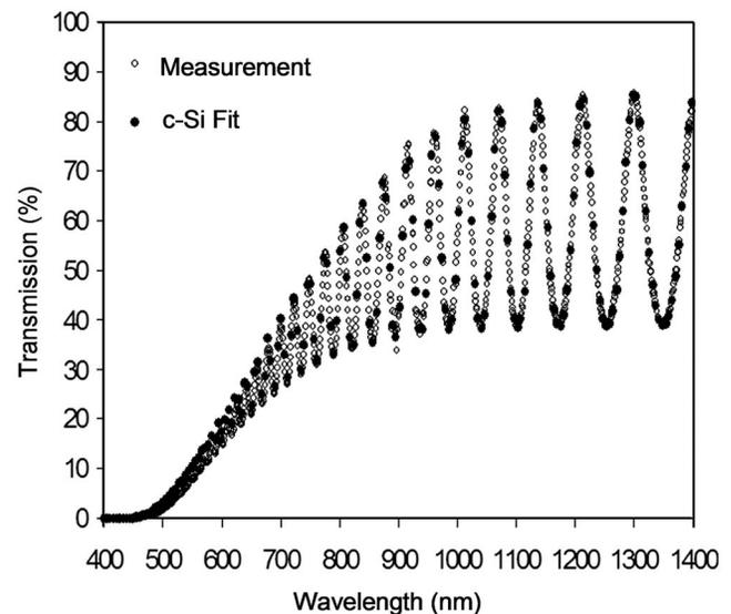
FIG. 6. Optical transmission spectrum of the EVA2 *n*-type base layer. The filled circles are a fit of transmission through this glass|*n* structure assuming single-crystal silicon optical properties for the *n*-layer. Fitted *n*-layer thickness is 2410 nm with 47 nm thickness variation.
