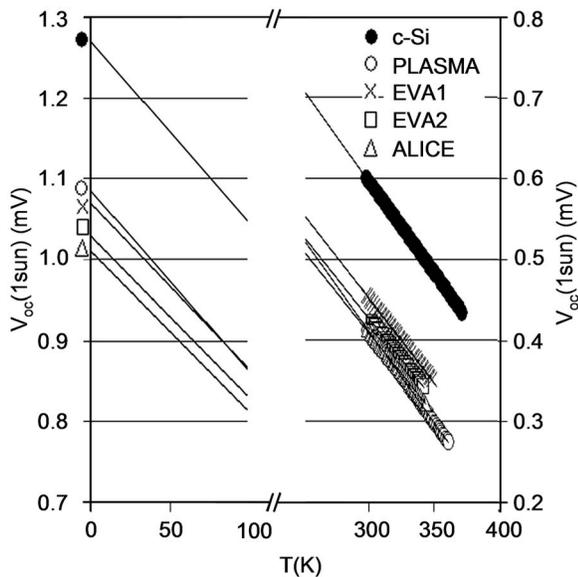
FIG. 7.  $V_{oc}(1 \text{ sun})$  of the poly-Si solar cells as a function of temperature compared to that of a single-crystal silicon solar cell. The straight lines extending from the data points are extrapolations.
