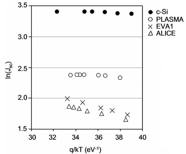
FIG. 5. Short-circuit current density ( $J_{sc}$ ) of the solar cells under the xenon lamp spectrum as a function of temperature.
