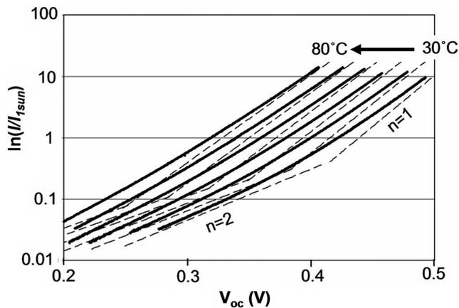
FIG. 3. Superposition of Suns- $V_{oc}$  curves of EVA2 from 30 to  $80^\circ\text{C}$ . For clarity, only six curves corresponding to  $10^\circ\text{C}$  increments are shown. The dashed lines represent the fits to the  $n=1$  and  $n=2$  recombination currents.
