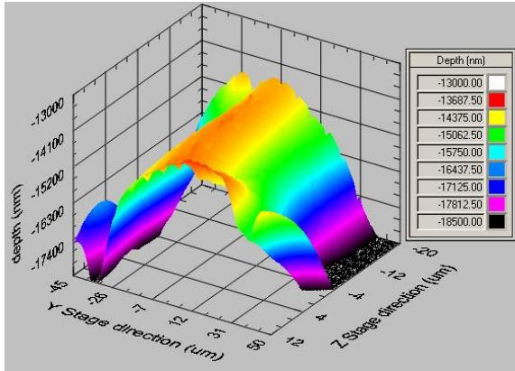
Fig. 2: Topographic slice of the flattened droplet.
