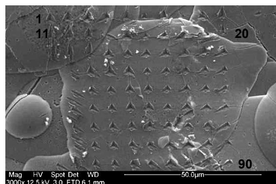
Fig. 1: An indented flattened solidified droplet with reference to specific indentations.
