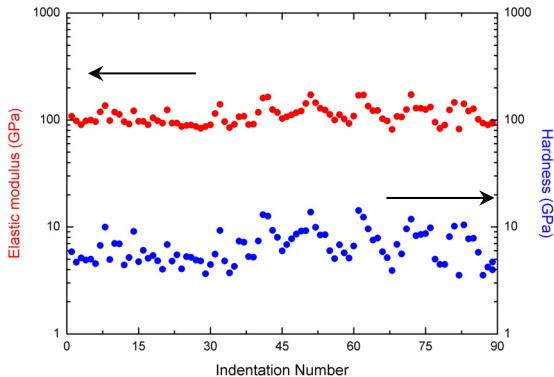
Fig. 3: Hardness and elastic modulus from indentations on the solidified flattened droplet.
