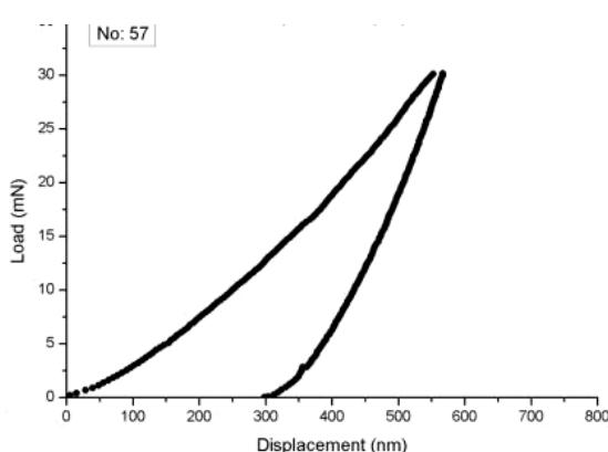
Fig. 4: Loading-unloading curves for an indentation (a) adjacent to a crack (indentation # 30), (b) on a sloped section (indentation # 83) and (c) on the top flat surface (indentation # 57).
