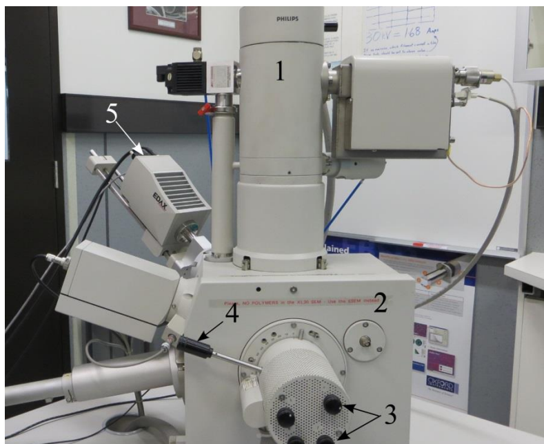
Figure 2-12 Philips XL30 SEM with EDAX attachment for EDS where numbers are indicating 1: electron column, 2: sample chamber, 3: stage controls, 4: stage tilt, and 5 EDS detector.
