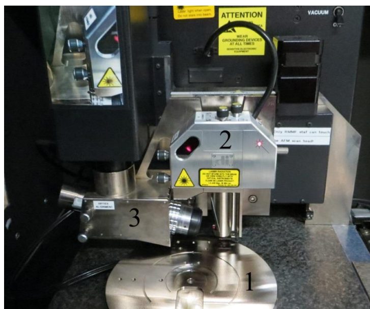
Figure 2-15 Nanoscope D3100 AFM in the RMMF where numbers are indicating 1: sample stage, 2: scanning head, and 3: optics for alignment.
