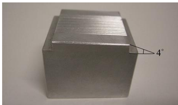
Figure 2-3 Aluminium block with channels used for mounting 25 mm length fibres. The mounting block base is at an angle of 4^\circ so that when the block is placed under the evaporation source, there is an angle of 86^\circ between the fibre tip and the source (see Section 3-2).
