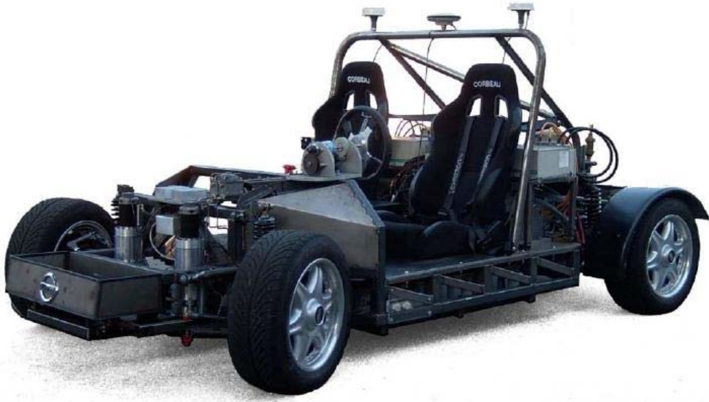
Figure 1.5: A Steer-by-Wire research vehicle [42].
